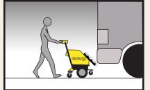
CarCaddy moves vehicles down production or assembly lines.
