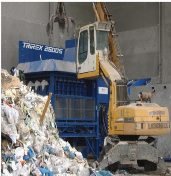
TRIREX 2600 S in construction and demolition waste
