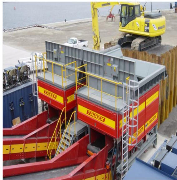
Two TRIREX 2600 S shredders on C&D waste
