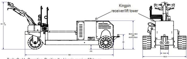
TrailerCaddy Operation: Position the kingpin receiver/lift tower directly below the kingpin of the trailer. Engage the hydraulic lift to rais the front end of the trailer off the ground. Press butterfly throttle control forward or backward to move trailer.
